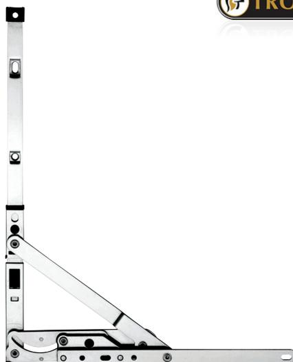
The Mega Egress Hinge is designed for use on casement window systems and is suitable for most side hung applications. Due to the superior integral strength, the hinge can be used for all sash widths up to 900mm with a maximum load of 40kg.
